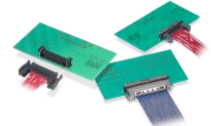
FX15 Wire-to-Board Pitch: 1.0mm Applicable Cable: 36~40 AWG (Thin Wire Coaxial Cable) 28~32 AWG (Discreet Cable) Rated Current: 0.5A No. of Pos.: 21,31,41,51
