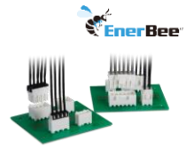
DF33C Pitch: 3.3mm No. of Pos.: 2-12 Rated Current: 5A Max.
