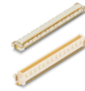
FX10 PCIe Gen.4 (16Gbps) Pitch: 0.5mm Mated Height: 4-8mm No. of Pos.: 80-168 Rated Current: 0.3A
